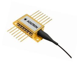
The 795nm series laser diodes are fabricated in a hermetically sealed 14-pin butterfly package. The laser diodes contain a monitor photodiode, thermoelectric cooler (TEC), and a thermistor to secure high-quality laser performance. Our laser products are Telcordia GR-468 qualified and in compliance with RoHS Directives.
